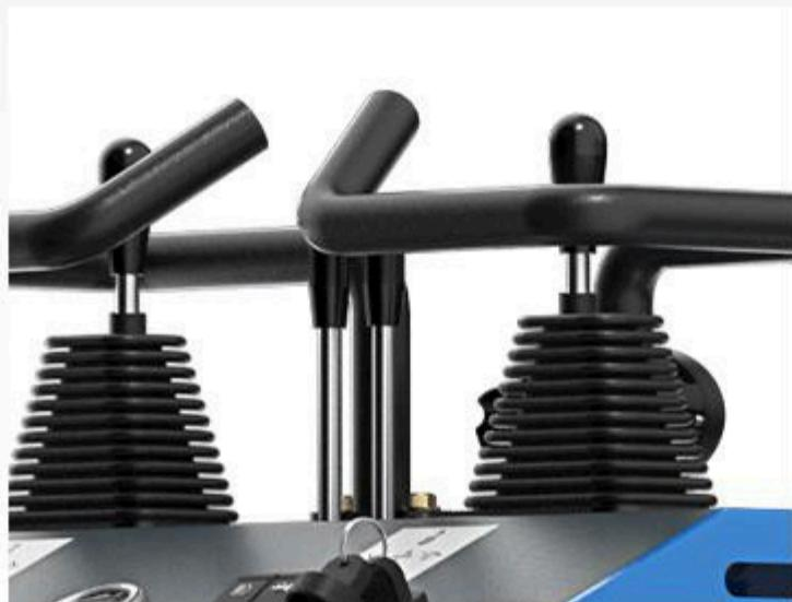
» The attachment operating lever provides precise hydraulic control, enabling efficient and flexible operation of various attachments.
