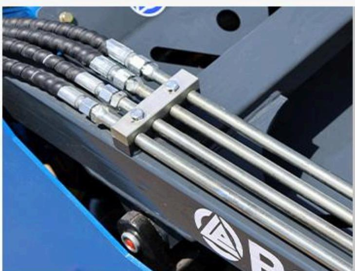
» A neatly arranged metal oil pipe runs above the robotic arm, ensuring durability and resistance to damage.
