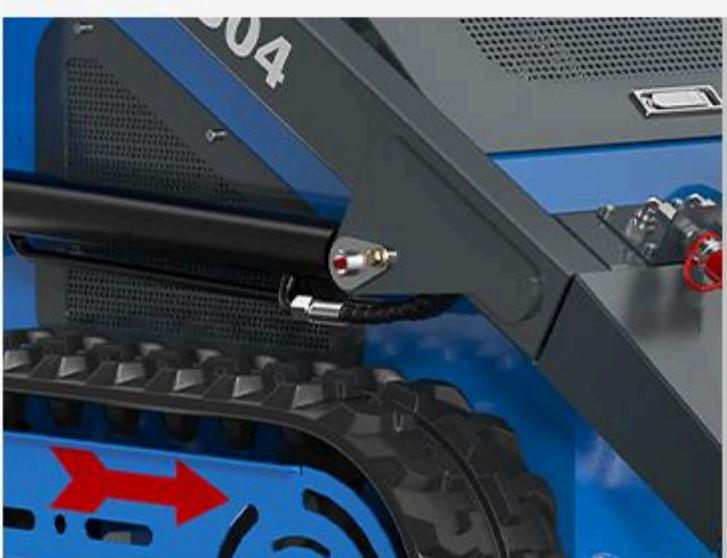
» The oil pipe adopts a built-in pipe arrangement, which can effectively protect the oil pipe, reduce wear and tear and prolong the service life of the oil pipe.
